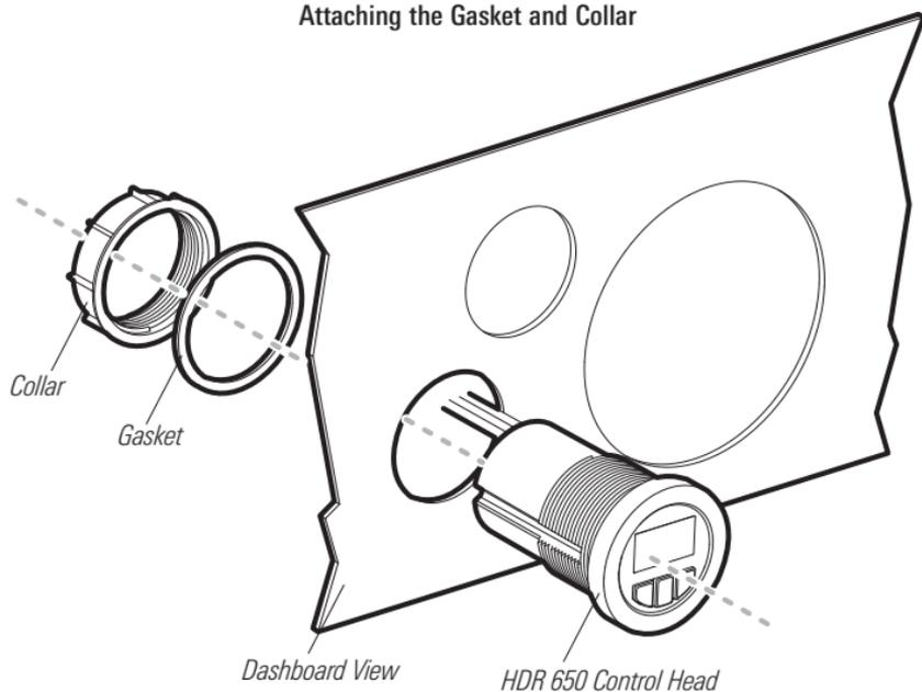
4. Hand-tighten the collar until the HDR is securely mounted in the dashboard. Make sure that the face of the HDR stays oriented upright.
