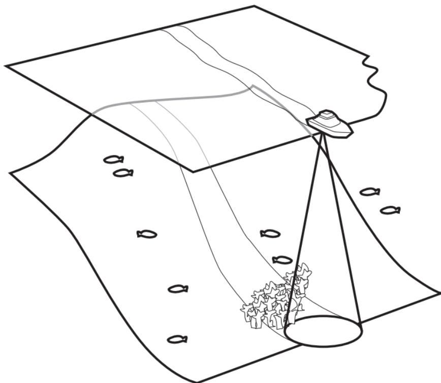
Sonar is very fast. A sound wave can travel from the surface to a depth of 240 ft (70 m) and back again in less than 1/4 of a second. It is unlikely that your boat can "outrun" this sonar signal.
