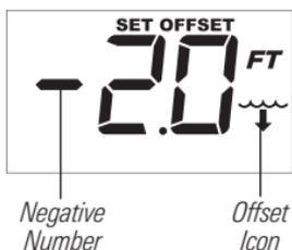
**Keel:** Press the DOWN arrow key to enter the measurement from step 1 as a negative (-) number. (-1 to -10 feet, -.1 to -3.0 meters, or -.1 to -1.6 fathoms; Default = 0)
