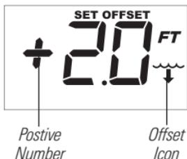
**Waterline:** Press the UP arrow key to enter the measurement from step 1 as a positive (+) number. (+1 to +10 feet, +.1 to +3.0 meters, or +.1 to +1.6 fathoms; Default = 0)
